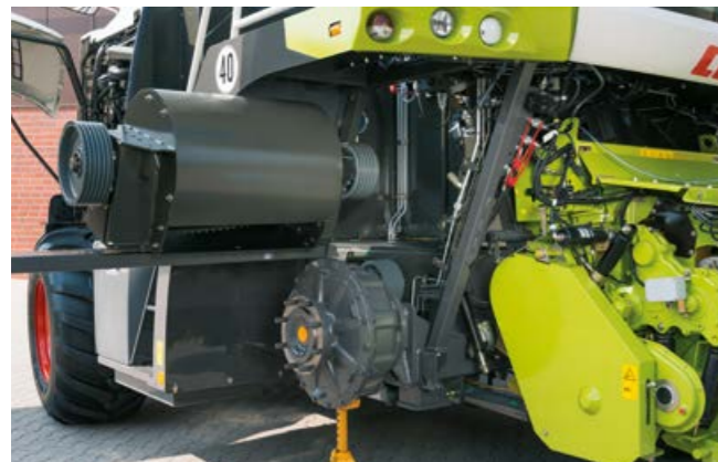
Easy removal and installation of the accelerator
