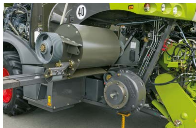
Easy removal and installation of the accelerator
