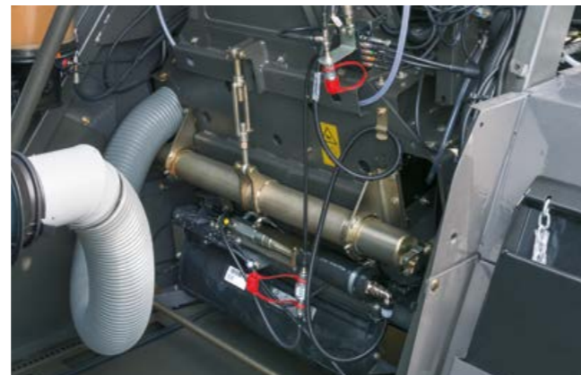
Mechanical adjustment of the crop accelerator clearance
