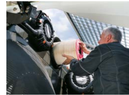
Air filter change without tools
