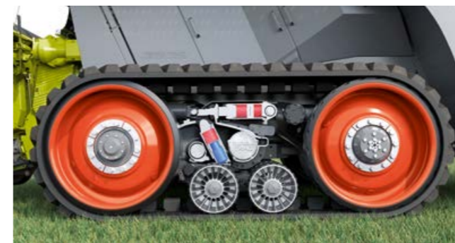
100% contact area: the track roller is in full contact with the ground.
