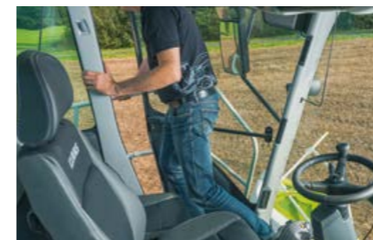
The seat contact switch automatically switches off the front attachment and main drive
