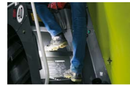
LED step lighting for safe access to the comfort cab
