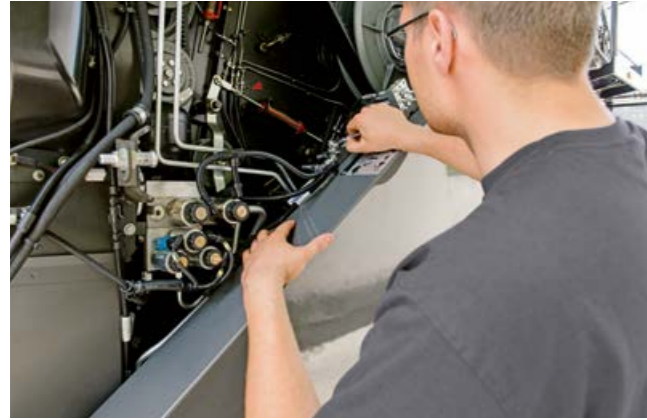
You can switch between the two speed ranges of the threshing drum speed reduction gearbox manually via a hydraulic valve.
