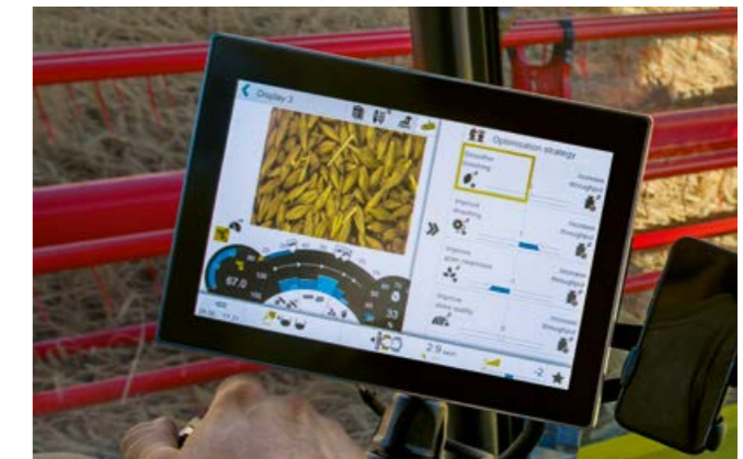
Intelligent control by CEMOS AUTOMATIC via CEBIS.
