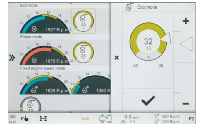
Engine droop setting for 'Eco' and 'Power', and for the engine speed memory.
