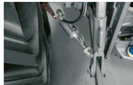
Optional hydraulic side stabilisers ensure greater safety and ease the work load
