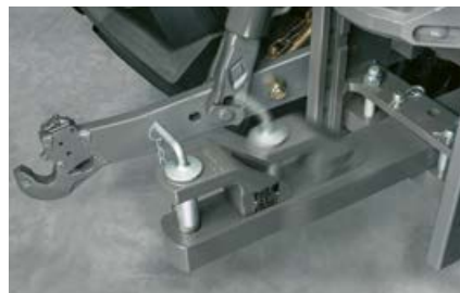
Several positions are available in the drawbar versions. The extended position increases manoeuvrability.
