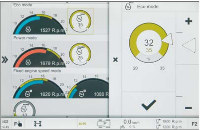
Engine droop setting for 'Eco' and 'Power', and for the engine speed memory.
