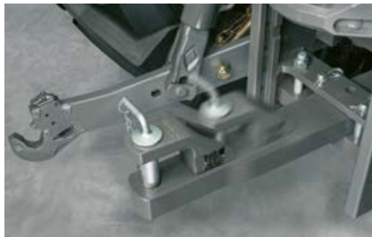
Several positions are available in the drawbar versions. The extended position improves manoeuvrability.
