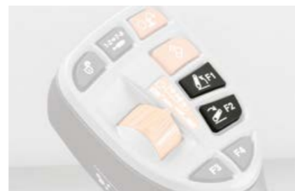
The rear linkage can be operated from the side console or the multifunction control lever.
